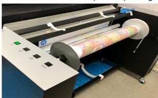
The versatility and high capacity of the Roll Wind Modules enables them to handle a wide variety of different print media, (for example, reflecting or transparent media), both in wind and unwind modes.
