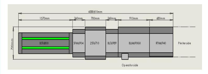
The system requires 400 mm of additional floor space at the front and rear side of the machine for installation, operation and maintenance.
