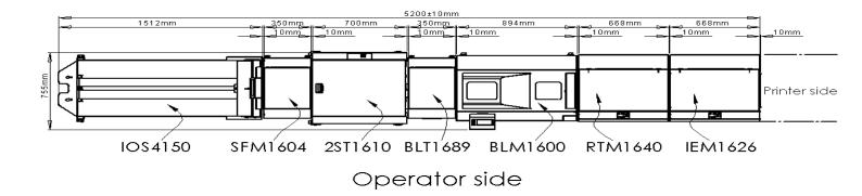
The system requires 400 mm of additional floor space at the front and rear side of the machine for installation, operation and maintenance.
